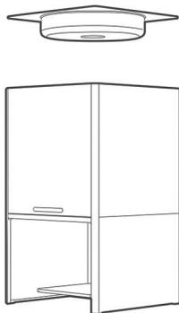
Fig. 9: Removing the top cover of the Buccaneer®.
